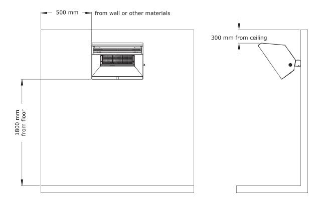
The heater discharges products of combustion from the top of the unit. If ceiling clearance is not maintained this could potentially be a fire hazard and surfaces may discolour.
