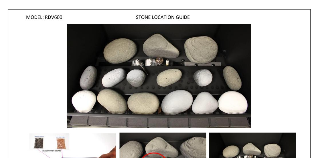
Mix the bag of Vermiculite to the bag of Glass and pour into the tray
