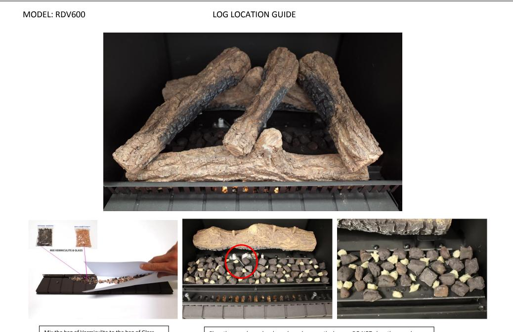
Mix the bag of Vermiculite to the bag of Glass and pour into the tray
