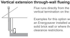
Flue runs directly from the unit to a vertical termination on the roof.
