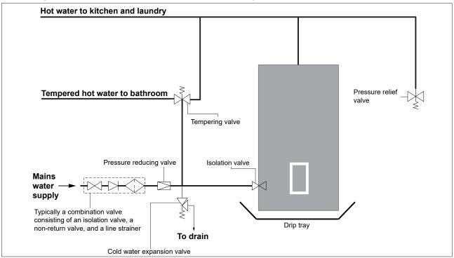
Plumbing setup for a low pressure stainless steel cylinder - open vented
